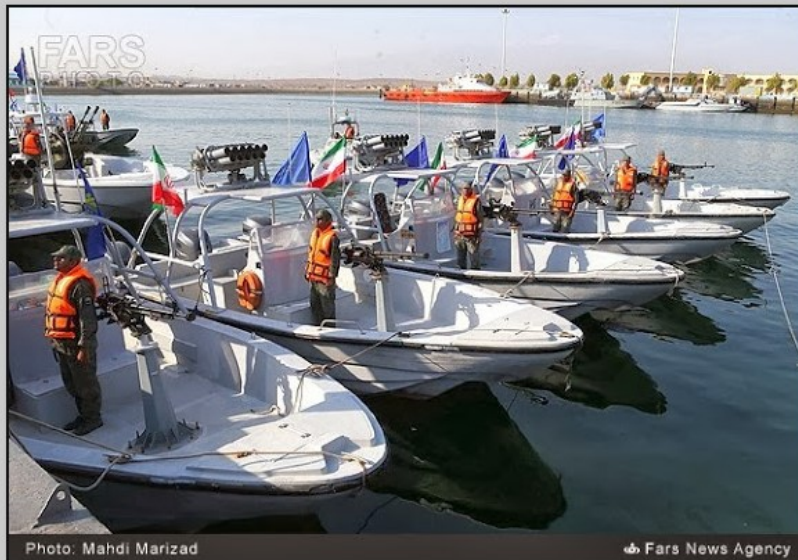
IRGC-N FB type MIL-40 inshore patrol boat armed with 107 mm MLRS and DShK 12.7 mm HMG
